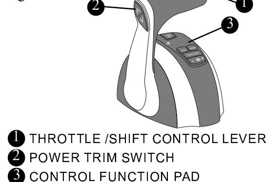
There is a “THROTTLE ONLY” button on the throttle control that when depressed will disengage the shifting mechanism and will allow you to operate the throttle without engaging the propeller. The button will automatically engage the shifting mechanism once the throttle control has been moved back to its center position.
