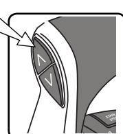
Use the trim switch to obtain an ideal boat angle (in relation to the water surface) for a given load and water condition. In most cases, best all around performance is obtained with the engine adjusted so that the boat will run at a 3° to 5° angle to the water.
