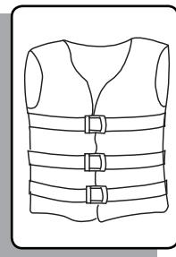
**Type III**, Flotation-aid Life vest is designed so that conscious wearers can turn face-up. Designed for comfort while engaged in water skiing or other forms of water activities.
