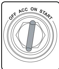
**ACC**= Power to instrument panel , gauges and other systems. No power to engine.
