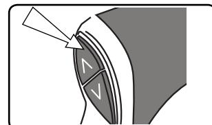
Use the trim switch to obtain an ideal boat angle (in relation to the water surface) for a given load and water condition. In most cases, best all around performance is obtained with the engine adjusted so that the boat will run at a 3° to 5° angle to the water.
