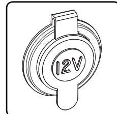
If equipped, the optional trolling motor panel also includes a 12V receptacle which provides accessory power at the bow of your boat.
