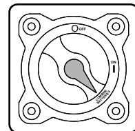
In the event a battery discharges completely, you will still be able to start the engines by turning the battery switch to the “COMBINE BATTERIES” position. This accesses the charged battery for engine start. After the engine starts, return the battery switch to the “ON” position until all batteries are charged.
