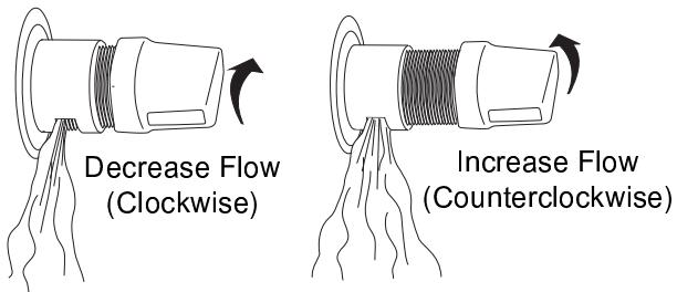
through the system. When not in use the standpipe can be stored in the clips on the underside of the livewell cover. A flow control valve (Figure 3.9.1) at the livewell water inlet controls the flow of water into the livewell. To increase the water flow, turn the valve counterclockwise. To decrease flow, turn the valve clockwise.
