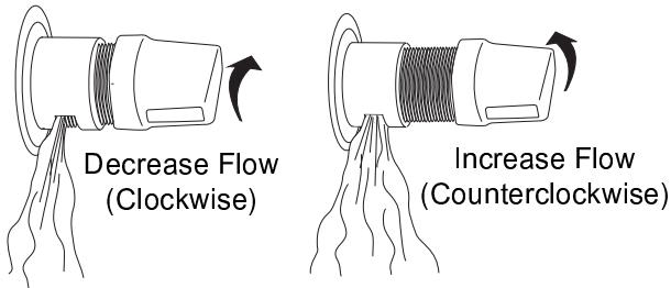
can be stored in the clips on the underside of the livewell cover. A flow control valve (Figure 3.9.1) at the livewell water inlet controls the flow of water into the livewell. To increase the water flow, turn the valve counterclockwise. To decrease flow, turn the valve clockwise.
