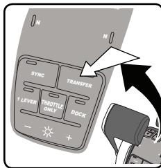
**NOTE:** Station transfer is cancelled if not completed within ten (10) seconds. Press and release the TRANSFER button again to re-initiate a station transfer.
