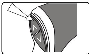
Use the trim switch to obtain an ideal boat angle (in relation to the water surface) for a given load and water condition. In most cases, best all around performance is obtained with the engine adjusted so that the boat will run at a 3° to 5° angle to the water.
