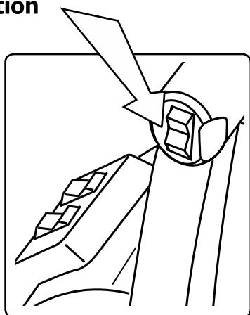
Use the trim switches to obtain an ideal boat angle (in relation to the water surface) for a given load and water condition.
