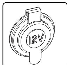
Your 230 Outrage is equipped with a 12 volt accessory receptacle located on the helm switch panel (See fig. 2.10.1). The DC receptacle is to be used with any 12 volt accessories using this style of plug.
