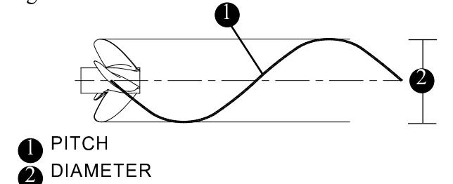
In general, changing to a lower pitch propeller will increase acceleration and load pulling capability, with a slight decrease in top end speed. If you choose to change propellers, the type should be discussed with your Boston Whaler® dealer. All propellers are designed to provide maximum forward thrust, consequently, the reverse thrust of the propeller will not be as efficient.
