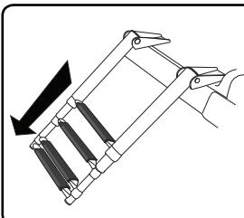
When not in use your swim ladder should be retracted and secured. To secure the ladder reverse the deployment method shown above.
