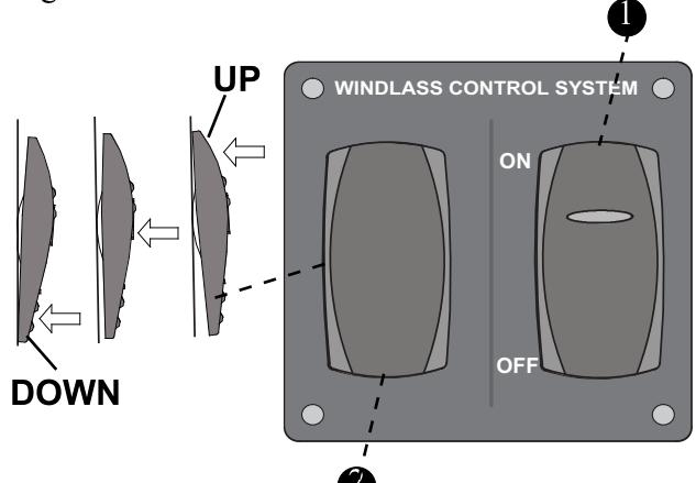
Activation of the windlass is controlled by a switch located to the left of the power switch. The activation switch is a momentary type switch, which means that there must be constant pressure applied to operate the anchor windlass and raise or lower the anchor.
