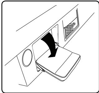
Simply lift up on the seat using the molded hand hold and pull away from the freeboard to drop down in a seated position.
