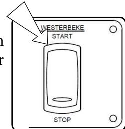
**DO NOT** crank the generator for more than 20 seconds at a time. Allow for a 60 second cool down period between cranking attempts.
