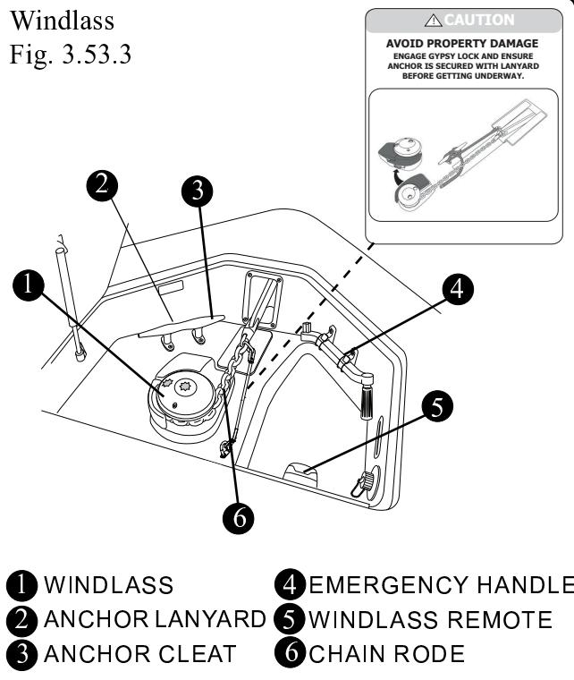
Be sure to attach the anchor lanyard when the anchor is stowed in the bow pulpit.
