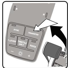
**NOTE:** Station transfer is cancelled if not completed within ten (10) seconds. Press and release the TRANSFER button again to re-initiate a station transfer.
