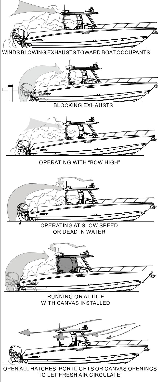
Dangerous concentrations of Carbon Monoxide will be present if the engine(s) exhaust system leaks OR insufficient fresh air is circulating.
