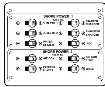
The single cord shore power scenario described in the previous column utilizes the generator to supplement power. Although this setup provides maximum voltage to your boat, you may find at times that the generator noise is too disruptive. You can still power your boat sufficiently by utilizing the breakers as follows:
