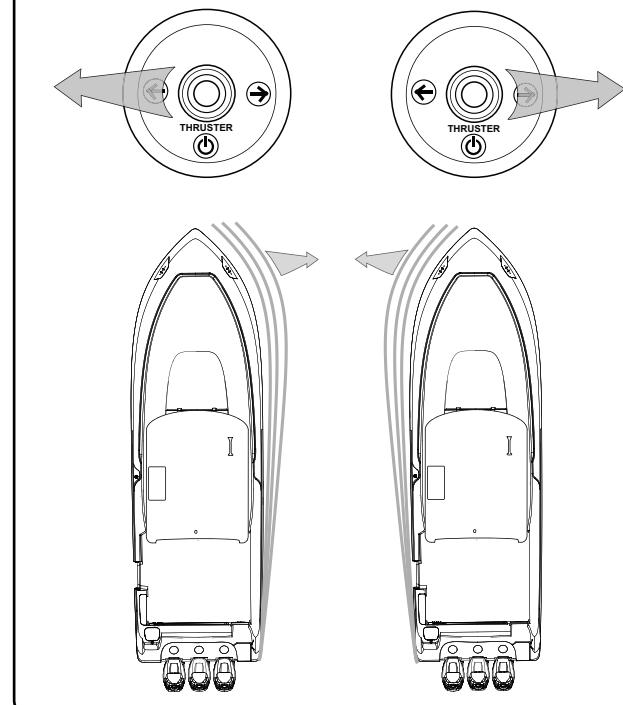
When the desired boat movement has been achieved return the joystick to the center position (spring return).
