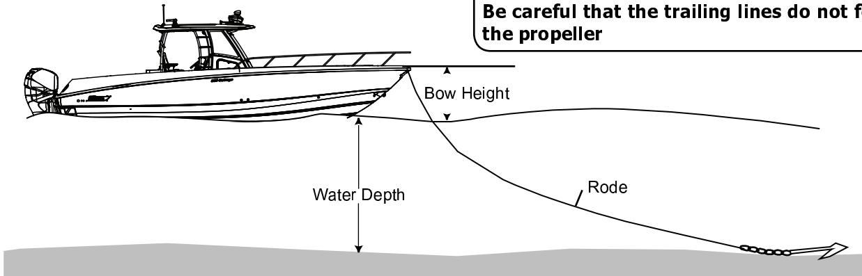
$$\text{Rode length} = (\text{bow height} + \text{water depth}) \times \text{Scope}$$
