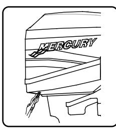
**NOTE:** If no water is coming out of the water pump outlet, stop the engine and check cooling water intake for obstructions. No obstruction may indicate a water pump failure or blockage in the cooling system. These conditions will cause the engine to overheat. Have the engine checked by your dealer. Operating the engine while overheated will cause engine damage.
