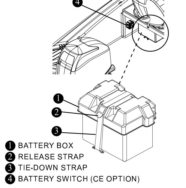
Before use, check the battery for loose connections or wiring. Normal maintenance should include:
