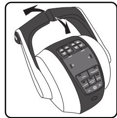
4. Adjust the control handles to the desired throttle and gear position.
