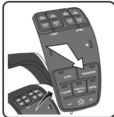
2. The lights will blink if the positions of the control handles are not aligned with the control handles at the station you are transferring from. Move the control handles until the blinking stops and the lights are solid.
