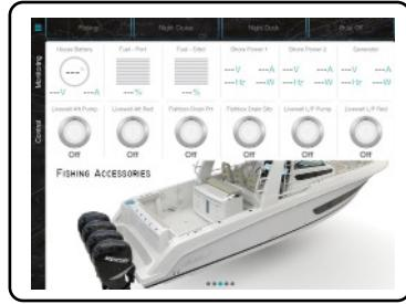
Next page gives the operator the ability to turn ON and OFF the bilge pumps, fresh water pump, washdown pump and discharge pump.
