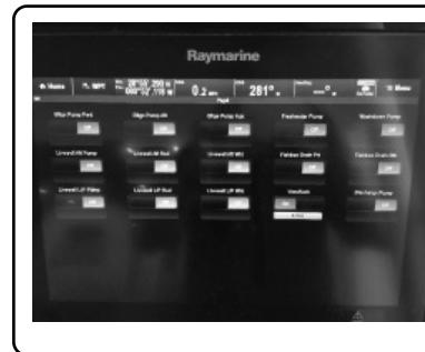
The various systems and components can be switched ON and/or OFF on the Raymarine interface by touching the selected component switch on the screen and dragging the icon to the right or left (See fig. 4.17.1).
