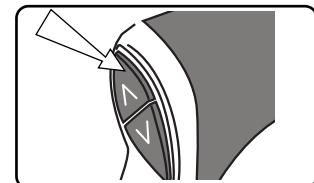
Use the trim switches to obtain an ideal boat angle (in relation to the water surface) for a given load and water condition.
