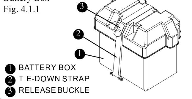
The battery box is located inside the console on the starboard side. Your battery should always be enclosed in the battery box provided with your boat.
