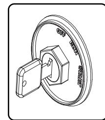
**RUN** = Power to instrument panels and gauges
