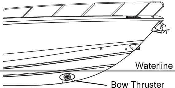
If equipped, the bow thruster joystick is located on the control station is used to operate the thruster and maneuver the bow of your boat.
