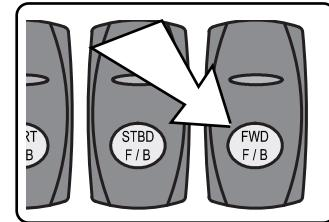
Check these breakers first and reset if a problem arises with the pumps failing to activate when the switches are depressed.
