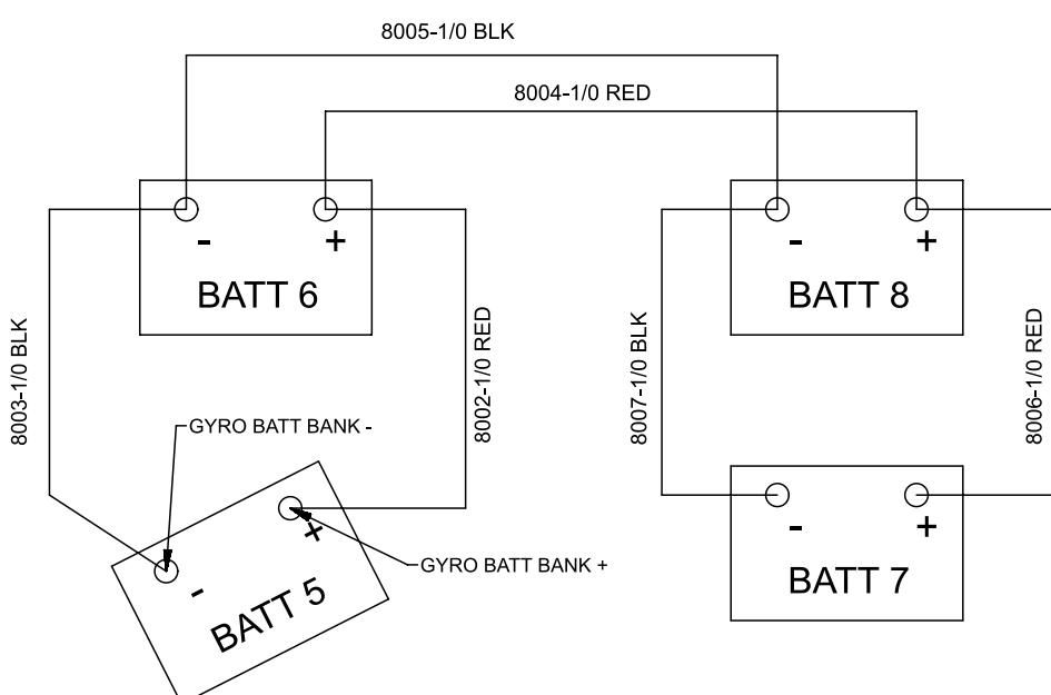
All battery jumper to be labeled on both ends according to this detail
