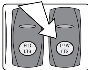
The underwater lights are powered by the "U/W LTS" switch on the helm switch panel (See fig. 2.17.1). The lights are protected by the "U/W LIGHTS" breaker on the main breaker panel located on the starboard gunnel opposite of the helm (See fig. 4.18.1).
