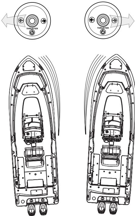
When the desired boat movement has been achieved return the joystick to the center position (spring return).
