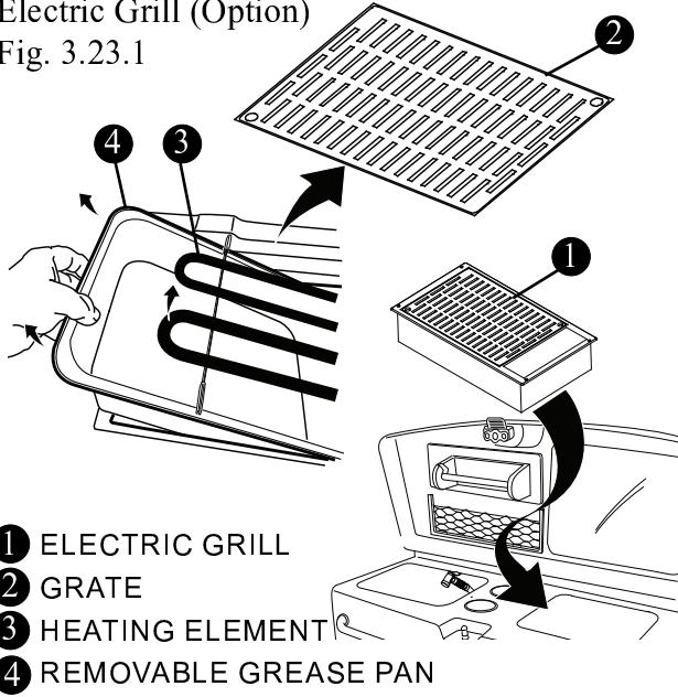
When replacing the pan, assure that it is completely contained within the grill and that the side of the pan does not extend outside of the grill sides.
