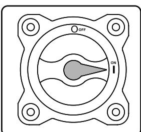
In the event a battery discharges completely, you will still be able to start the engines by turning the engines switch to the “COMBINE BATTERIES” position. This accesses the charged battery for engine start. After the engine starts, return the battery switch to the “ON” position until all batteries are charged.
