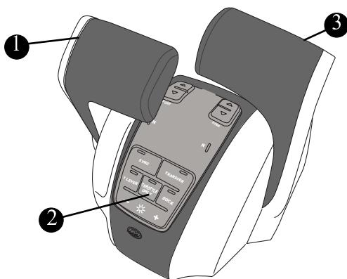
1 PORT ENGINE GEAR SHIFT/THROTTLE
