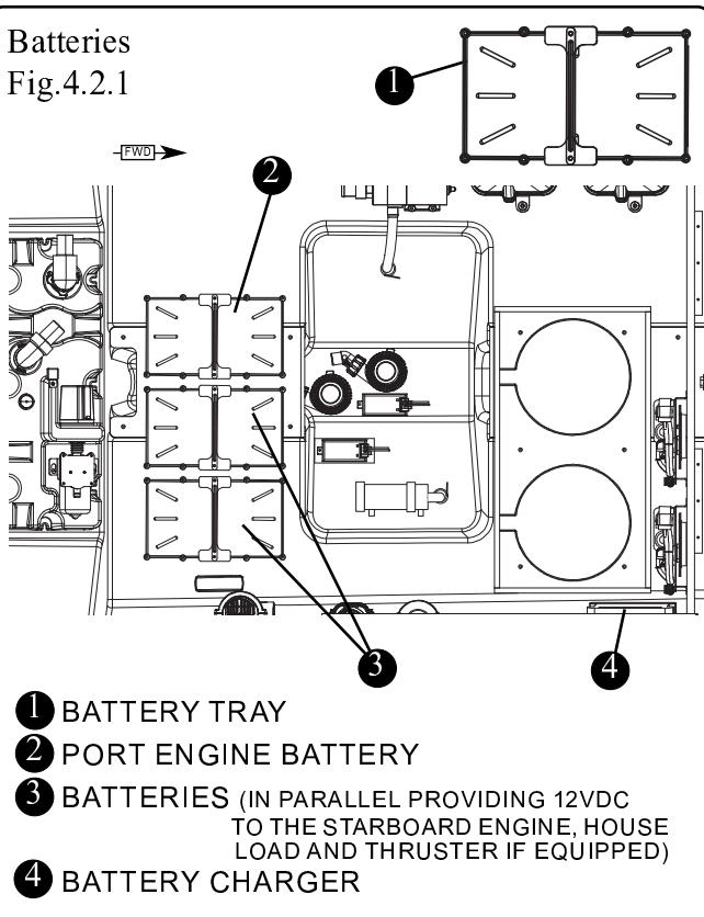
Before use, check each battery and the charging system for loose connections or wiring. Normal maintenance should include:
