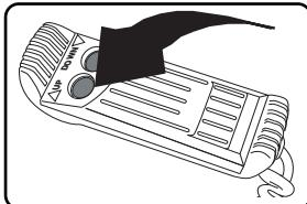
The anchor windlass can be operated from the bow with the use of the windlass remote which is stowed in the bow locker.
