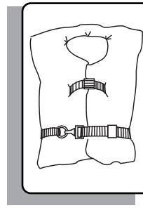
**Type II**, Near-shore Life Vest, "keyhole" vest with flotation filled head and neck support is also designed to turn a person face up, but the turning action is not as pronounced. Use in calm inland waters or where quick rescue is likely.
