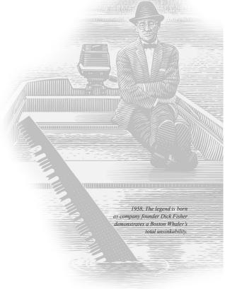
In 1958, company founder Richard T. Fisher introduced the first Boston Whaler® boat in Braintree, Massachusetts. It featured two significant innovations: first, its twin sponson hull design produced superior stability and a remarkably dry ride; second, its unique foam core construction made the boat not only durable, but unsinkable as well.
