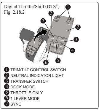
The 285 Conquest is equipped with a state of the art "drive-by-wire" gear shift and throttle control system. The Digital Throttle/Shift (DTS®) is the latest technology in recreational boating. Located on the console, starboard of the helm (See figure 2.8.2). The gear shift/throttle control unit controls both the shifting mechanism and throttle.
