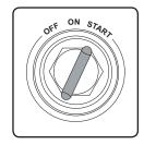
When engine starts, release key. The key will return to the "ON" position.
