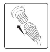
• Turn the forward portion of the plug clockwise to lock.
