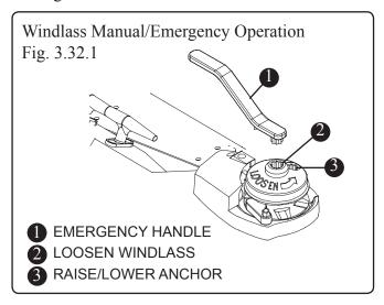
windlass chainwheel. The star socket located offcenter is used for retrieving and lowering the anchor. Turning the handle counterclockwise will allow you to lower the anchor, while turning it clockwise will raise it.
