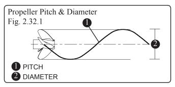
In general, changing to a lower pitch propeller will increase acceleration and load pulling capability, with a slight decrease in top end speed. If you choose to change propellers, the type should be discussed with your Boston Whaler® dealer. All propellers are designed to provide maximum forward thrust, consequently, the reverse thrust of the propeller will not be as efficient.
