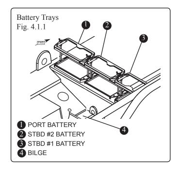
enclosure on the port side of the mid cabin. The batteries can be installed or removed by loosening the wing nuts and removing the retaining lid on the battery tray.
