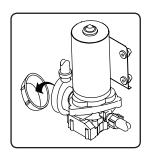
The raw water pump can be accessed through the aft cockpit deck hatch.
