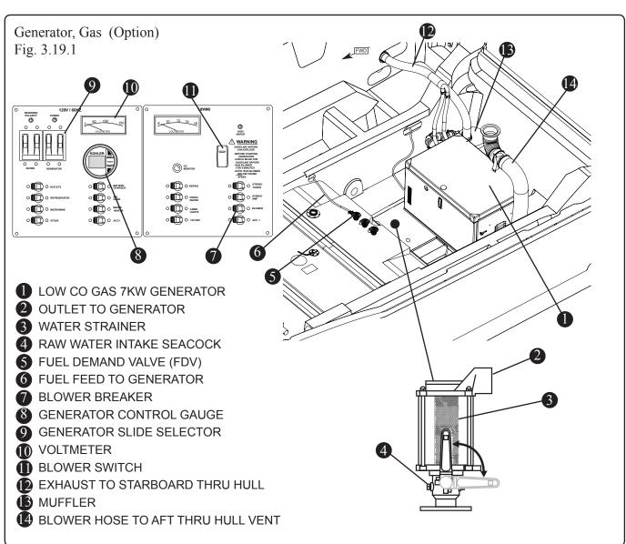
The generator draws fuel from the main fuel tank. The generator fuel system is designed to run out of fuel with about 1/4 tank of fuel remaining, leaving a reserve of fuel for the propulsion engines.
