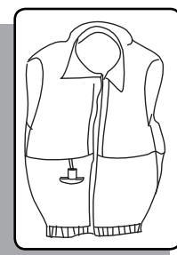
**Type V**, Special-Use devices, sailboat harnesses, white water vests, float coats, and hybrid vests which have minimum inherent buoyancy and an inflatable chamber.
