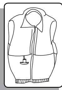
**Type V**, Special-Use devices, sailboat harnesses, white water vests, float coats, and hybrid vests which have minimum inherent buoyancy and an inflatable chamber.
