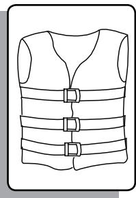
**Type III**, Flotation-aid Life vest is designed so that conscious wearers can turn face-up. Often designed for comfort while engaged in water skiing or other forms of water activities.
