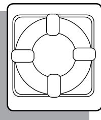
**Type IV**, Throwaway Devices, horseshoe buoys, ring buoys and buoyant cushions are designed to be grasped, not worn.
