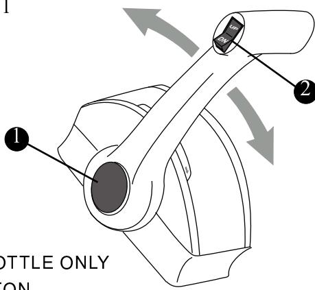
To reverse power, bring the control lever back to engage the reverse gear and increase the reverse thrust. The throttle control regulates the RPM of the engine. Regulating the RPM of the engine will control the speed of the boat.
