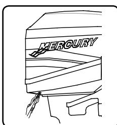
**NOTE:** If no water is coming out of the water pump outlet, stop the engine and check cooling water intake for obstructions. No obstruction may indicate a water pump failure or blockage in the cooling system. These conditions will cause the engine to overheat. Have the engine checked by your dealer. Operating the engine while overheated will cause engine damage.
