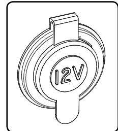
Be sure to use accessories that do not exceed the rated capacity of the circuit, (15 amps). Doing so will cause the in-line fuse to trip.
