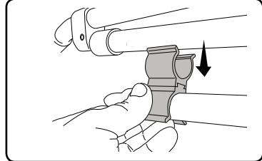
NOTE: Before attaching the straps, twist the straps a couple of turns to reduce noise from vibration when making way.
