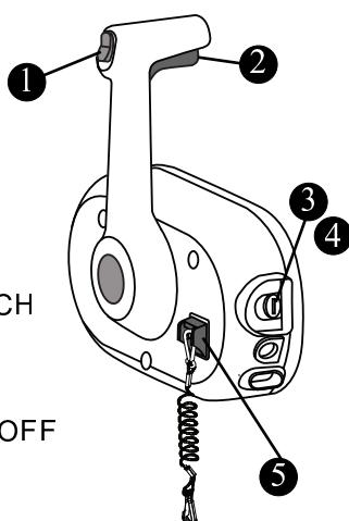
To reverse power, bring the control lever back to engage the reverse gear and increase the reverse thrust. The throttle control regulates the RPM of the engine. Regulating the RPM of the engine will control the speed of the boat.
