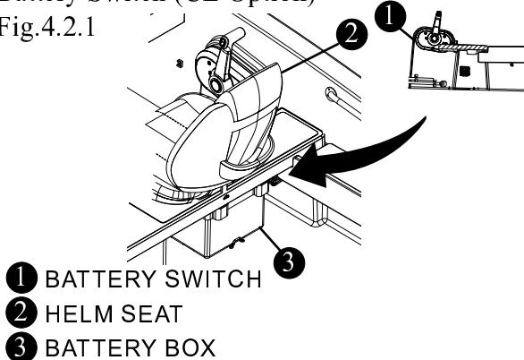
Your battery selector switch has two settings, "ON" and "OFF", "ON" gives you power from the battery.. "OFF" you have no power to the engine.
