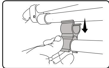
NOTE: Before attaching the straps, twist the straps a couple of turns to reduce noise from vibration when making way.
