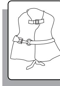
**Type I**, Off-shore Life Jacket is considered the most buoyant, it is designed to turn an unconscious person face up. Use in all types of waters where rescue may be slow, particularly in cold or rough water conditions.
