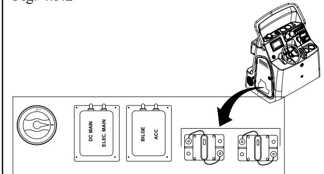
The trolling motor receptacle located at the bow of your boat is protected by a 40 amp breaker located on the forward wall of the console interior. There are two breakers, one each for the 12V or 24V trolling motor system.
