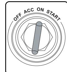
**ACC** = Power to instrument panel, gauges and other systems. No power to engine.
