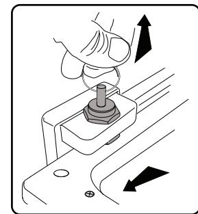
To unlock the cooler base, pull the locking pin up.
