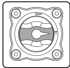
When leaving the boat for an extended period of time, turn the switch to the “OFF” position to avoid discharging the batteries.
