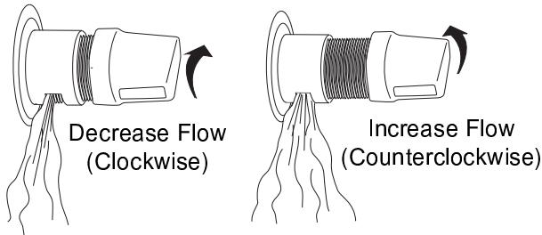
livewell cover. A flow control valve (Figure 3.11.1) at the livewell water inlet controls the flow of water into the livewell. To increase the water flow, turn the valve counterclockwise. To decrease flow, turn the valve clockwise.
