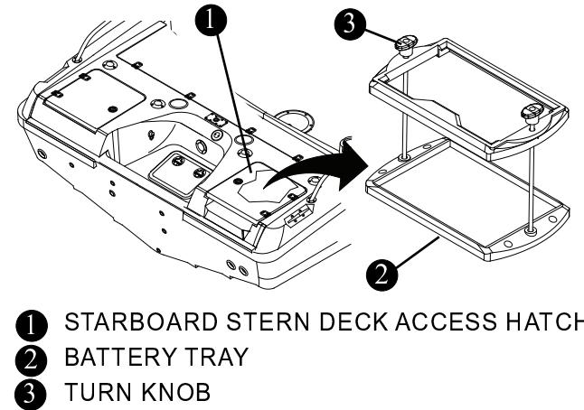
The battery should always be kept in the battery tray provided with your boat. The tray is located in the starboard stern deck and can be accessed through the starboard stern deck access hatch.
