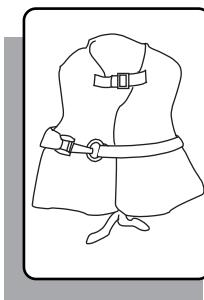
**Type I**, Off-shore Life Jacket is considered the most buoyant, it is designed to turn an unconscious person face up. Use in all types of waters where rescue may be slow, particularly in cold or rough water conditions.
