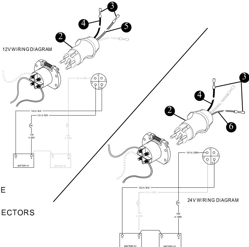
Each system (12V & 24V) is protected by a 40 amp breaker located at the bottom aft in the center console (Figure 4.3.2).
