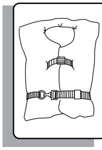
**Type II**, Near-shore Life Vest, "keyhole" vest with flotation filled head and neck support is also designed to turn a person face up, but the turning action is not as pronounced. Use in calm inland waters or where quick rescue is likely.
