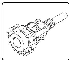
Turn clockwise to lock and thread the locking ring onto the receptacle to prevent accidental unplugging.
