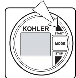
DO NOT crank the generator for more than 20 seconds at a time. Allow for a 60 second cool down period between cranking attempts.
