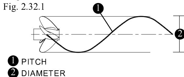
In general, changing to a lower pitch propeller will increase acceleration and load pulling capability, with a slight decrease in top end speed. If you choose to change propellers, the type should be discussed with your Boston Whaler® dealer. All propellers are designed to provide maximum forward thrust, consequently, the reverse thrust of the propeller will not be as efficient.
