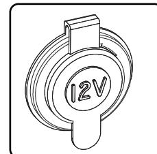
There is a 10 amp breaker located on the DC Main Distribution Panel (See figure 4.5.1). **Be sure to use accessories that do not exceed the rated capacity of the circuit, (10 amps) or the breaker will trip.**
