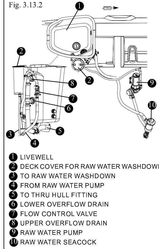
You can regulate the amount of water in the livewell by inserting the second drain plug (supplied) into the lower overflow drain thus raising the level of water to the upper overflow drain.
