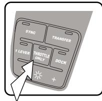
The button will automatically engage the shifting mechanism once the throttle control has been moved back to its center position.
