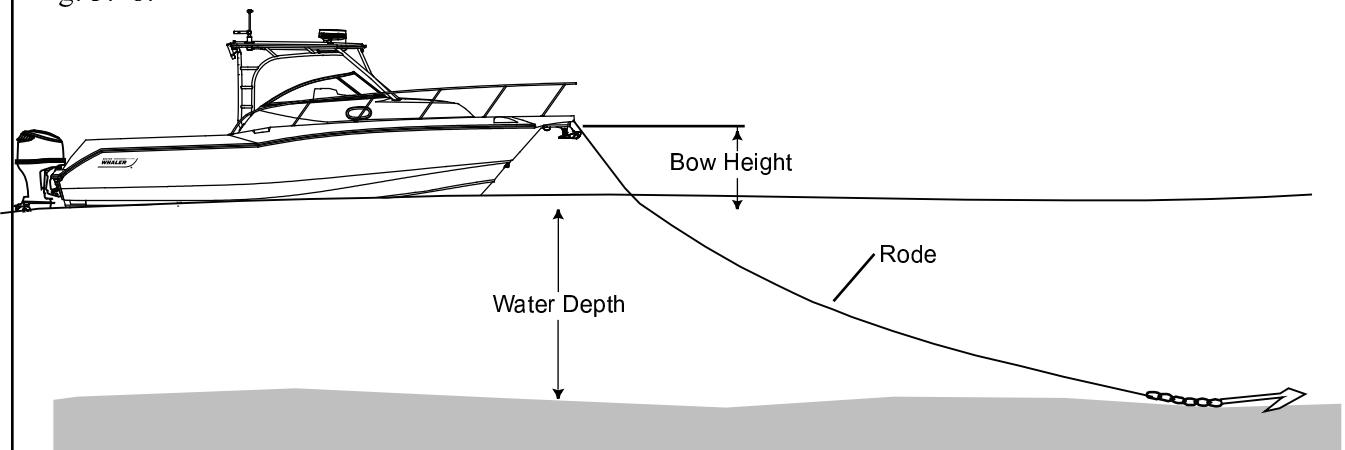
$$\text{Rode length} = (\text{bow height} + \text{water depth}) \times \text{Scope}$$
