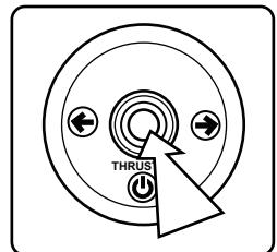
When the desired boat movement has been achieved return the joystick to the center position (spring return).
